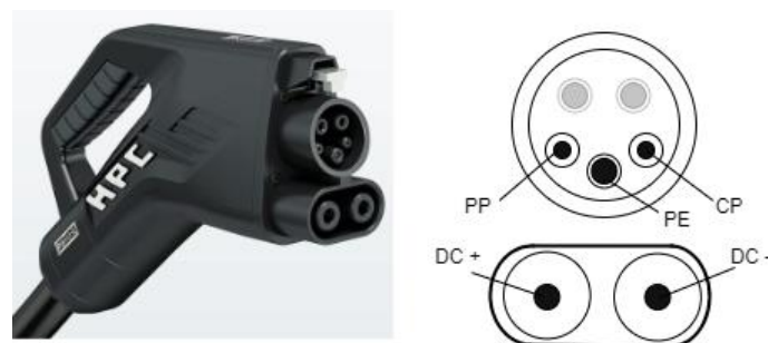
Fig. 5.29 CCS 1 DC charging plug and pin descriptions [10]
